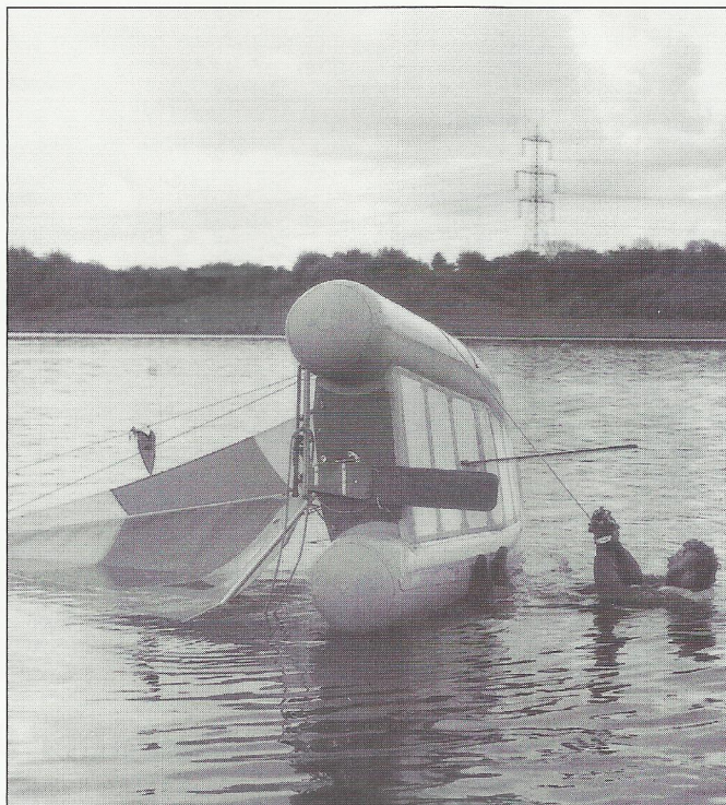
Boat almost upright using the short jib sheet – difficult to reach, though
